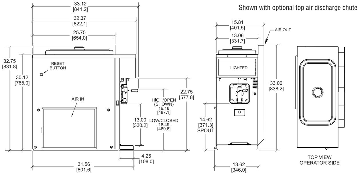
NOTE: FIGURES IN PARENTHESES INDICATE MILLIMETERS. / ALL DIMENSIONS PLUS OR MINUS 1/16 inch [1.5mm].
